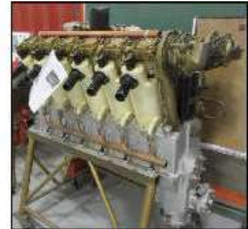
The V-12 Liberty engine was used in tanks, as well as WWI aircraft.
